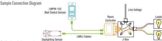
Plug DLM local network components together in any configuration using Cat 5e cables with RJ45 connectors.
