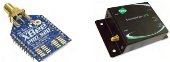
The ZigBee products for wireless connectivity enable either a wireless mesh network between multiple inverters at a site, or a wireless link between a master inverter and a remote internet gateway point.
