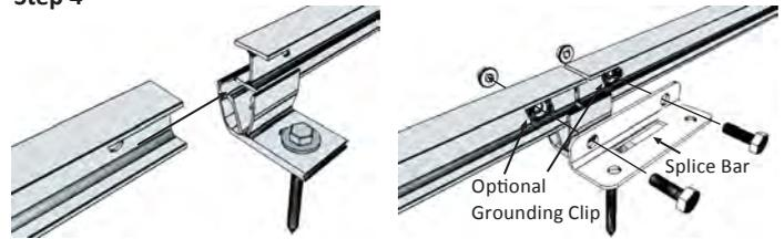
Remember to slide all mid-clamps into place prior to splicing.
