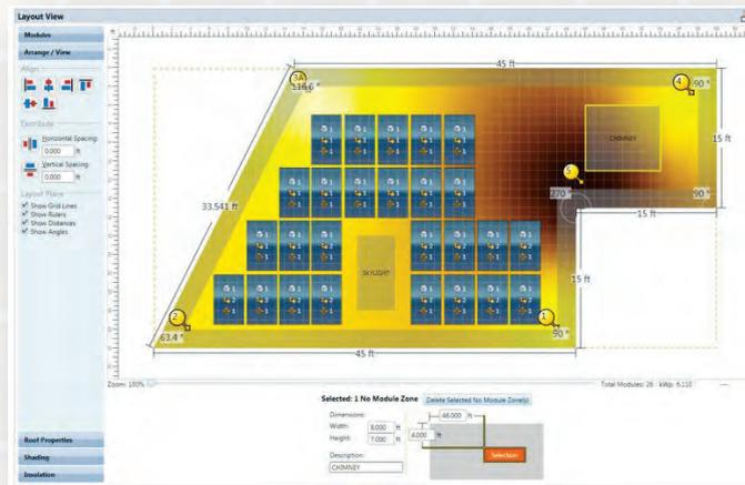
Lay out modules and estimate PV production with PV Designer™ software.
