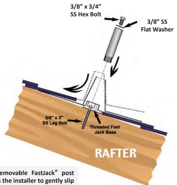
The removable FastJack® post allows the installer to gently slip the flashing over the base and under the delicate composition shingles.
