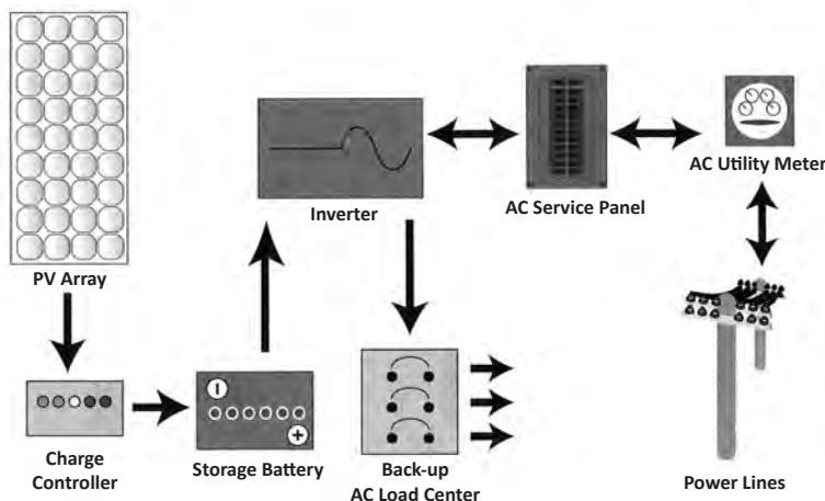
GRID-TIED SYSTEM WITH BATTERIES
