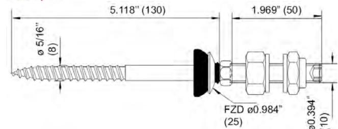
**IMPORTANT NOTE:** Metric drill diameters are necessary for optimal holding/clamping characteristics! Metric drills have to be used to not void the warranty. Refer to the US Assembly Instructions for EJOT Solar Fastenings or the installation manual to determine the appropriate pre-drill diameter for your specific project.
