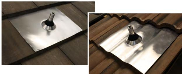
The QBase Universal Tile Mount is comprised of all aluminum stand off and flashing. All hardware is included. The tile is removed, the stand off is bolted into the rafter, and the tile is cut to allow for the stand off to pass through. An additional aluminum primary flashing is included for waterproofing at the sub-roof underlayment level. The aluminum flashing is then placed and molded to the shape of the tiles. This product can be installed on curved and flat tile roofs.
