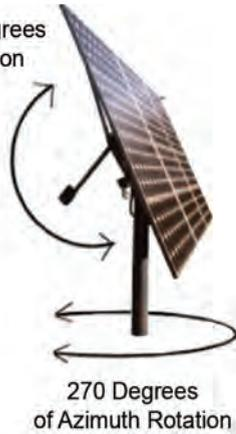
Compared to passive, tilt and roll trackers, azimuth trackers provide greater stability for large arrays. The corners do not protrude down towards the ground or stick up in the air to catch the wind. The bottom edge of the array always remains parallel to the ground and requires less ground clearance than tilt & roll designs. Wattsun Solar Trackers are available in five different sizes all manufactured in the USA.
