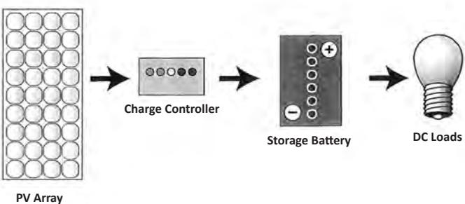
DC SYSTEM WITH BATTERIES
