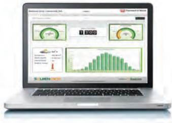
The required hardware comes standard and fully-integrated within all commercial and SMARTGRID inverters. A stand alone version is available for residential use with LCD or LITE gateway systems. The complete SolrenView system features inverter direct monitoring, revenue grade monitoring, agency reporting, SolZone sub-array current monitoring, a Kiosk View (flash view) and a weather station.
