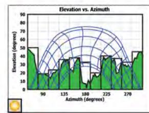
Alternative data views include monthly solar access and obstruction elevation vs. azimuth.
