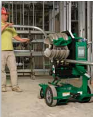
855GX - Complete with EMT/IMC/Rigid Bending Shoe Group
