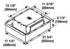
**10-Gang Fire Classified Floor Box** – Pre-assembled installation ready floor box has been designed to be installed in above grade concrete floors while maintaining the fire classification of the floor. This box is classified to be used in 1-, 1 1/2-, 2-, or 3-hour fire rated floors. Designed to accept standard size wall plates. **Box comes complete with all components needed for initiainstallation.**
