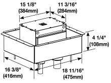
**4- & 5-Gang Fire Classified Floor Box** – Pre-assembled installation ready floor box has been designed to be installed in above grade (second floors and above) concrete floors while maintaining the fire classification of the floor. This box is classified to be used in 1-, 1 1/2-, 2- or 3-hour fire rated floors. Designed to accept standard size wall plates. **Box comes complete with all components needed for initial installation.**
