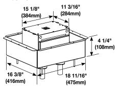
**4- & 5-Gang Fire Classified Floor Box** – Pre-assembled installation ready floor box has been designed to be installed in above grade (second floors and above) concrete floors while maintaining the fire classification of the floor. This box is classified to be used in 2-hour fire rated floors. Designed to accept standard size wall plates. **Box comes complete with all components needed for initial installation.**
