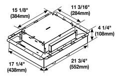
**6-Gang Fire Classified Floor Box** – Pre-assembled installation ready floor box has been designed to be installed in above grade concrete floors while maintaining the fire classification of the floor. This box is classified to be used in the 2-hour fire rated floors. Designed to accept standard size wall plates. **Box comes complete** with all components needed for initial installation.
