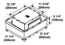
**10-Gang Fire Classified Floor Box** – Pre-assembled installation ready floor box has been designed to be installed in above grade concrete floors while maintaining the fire classification of the floor. This box is classified to be used in 2-hour fire rated floors. Designed to accept standard size wall plates. **Box comes complete with all components needed for initial installation.**
