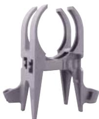
The ENT Support Unit (ESU) is designed to raise the tubing or conduit up off the concrete form during the concrete pour maintaining a level raceway. With its minimal surface contact, the ESU allows for maximum aggregate flow and concrete consolidation.
