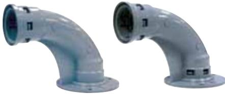
Both styles of stub down fittings are designed for direct connection to ENT on the horizontal by means of our unique six locking tab for concrete encasement Kwikon connection. The flanged base of the threaded 90° stub down offers contractors a NPSC threaded hub connection on the vertical – at the exit point of the slab, allowing for the direct transition to other raceway products.
