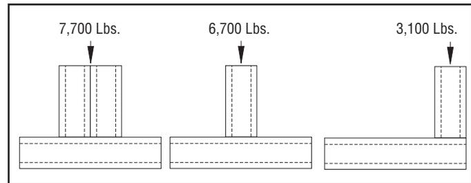
Resistance to Slip – 1,500 lbs. per bolt when 1/2" PS NS channel nuts are used.
