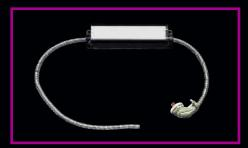
Emergency battery back-up ballast for Compact Fluoresecent Fixtures with (1) 13W-42W, (2) 13W-42W 4 Pin lamps, 120V or 277V electronic J box mount
