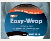
High quality unvulcanized rubber that will bond quickly to itself to form a solid mass of watertight protection. Self fusing with liner. Can be used as primary insulation for electrical wires and cable splices up to 600 volts. Conforms to irregular shapes and is flexible to withstand expansion and contraction. Highly resistant to salt water, steam, oils, detergents
