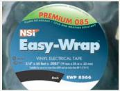
Premium 085 Easy Wrap is a 8.5 mil, all weather, premium grade, pressure sensitive vinyl electrical tape. Cold and sunlight resistant. Flame retardant. Suitable for use in all kinds of electrical and mechanical applications. Provides exceptional flexibility and performance over a wide range of temperatures. Available in standard black only. Suitable for use at no more than 600 V and not more than 80°C (176°F). CSA temperature range: -18°C to 105°C. Meets MIL-I-24391C, HH-I-595C and ASTM D-3005.
