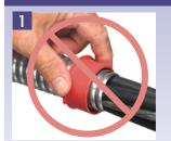
If you are using an end stop bushing, determine which one to use by sizing it to the cable bundle (not the metal jacket). Incorrect size shown above. The metal jacket should never go through the end stop.
