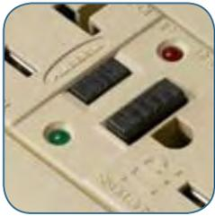
This patented industrial design includes an exclusive tamper resistant system to protect against objects being placed in a blade opening. Due to a unique switching technology, power is not present if an object is inserted within an individual slot. This is significantly superior to the plastic shutter method that is used by competition today.
