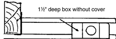
Foot straightened gauges for 1 1/2" deep box with cover or 2 1/4" deep box without cover. With foot broken off gauges for shallow pan box.
