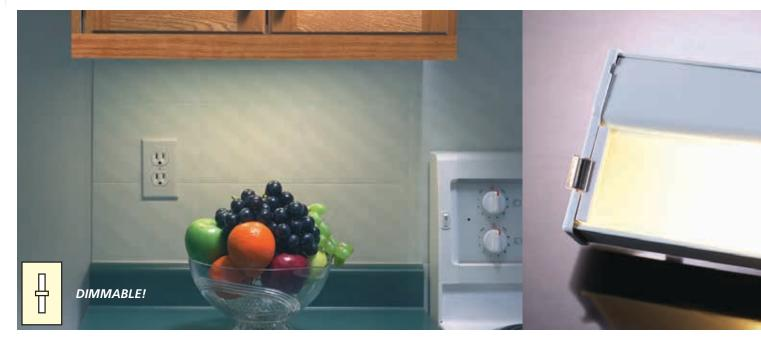
Xenon Task Light (XTL) is the perfect affordable solution for under cabinet, counter and shelf lighting. XTL utilizes an 18 watt xenon lamp that provides a better quality light (color rendering index RA = 100 and color temperature of 2750 Kelvin), longer lamp life (10,000 hours) and a cooler burning lamp when compared to traditional halogen products.
