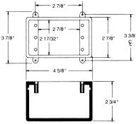
For terminations where hub requirements vary according to application – hubs easily made with flared wood bit or hole saw.
