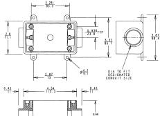
For through terminations where large devices or additional wiring capacity is required.
