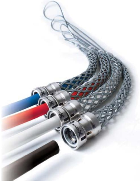
Dual lock pulling system using both a cam lock head and a double braided wire to quickly secure cable to rope without the fear of losing a conductor.
