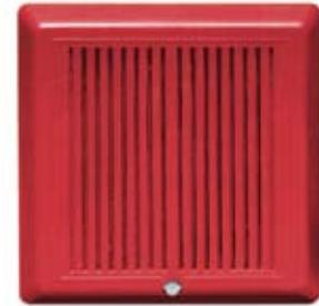
Edwards 2400 Series temporal horns and temporal horn-strobes are designed for use with compatible life safety communication and control equipment to alert occupants of a life safety event. The horn emits up to a 95dB (@ 1meter) low frequency sound, and must be connected to signal circuits that output a constant (not pulsed) voltage. A diode is used to allow full signal circuit supervision.
