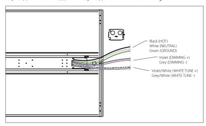
SpectraSync tunable white luminaires are provided with (2) 0-10V circuits. The violet and grey circuit is for wiring to any qualified 0-10V controller for dimming. The violet/white and grey/white circuit is for wiring to any qualified 0-10V controller for tunable white CCT control.
