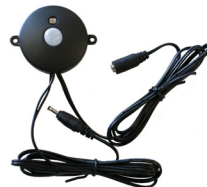
UCSENS-PIR PIR motion sensor, auto on/off with movement, max 24 watt in 12V or 36 watt in 24V, 6.4 ft. range
