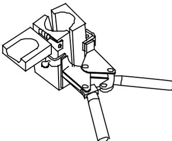
A semi-permanent graphite mold is used for making most CADWELD Connections. The mold controls the direction and speed of the molten CADWELD weld metal flow and its final shape. The graphite used in a CADWELD mold is a high temperature type that lasts for an average of 50 or more CADWELD connections under normal usage.
