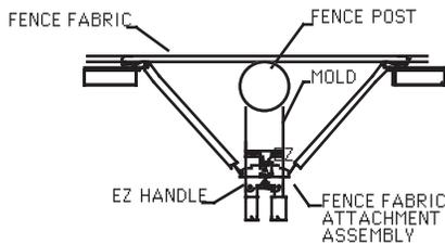
An easy to use, labor saving, Fence Fabric Attachment Assembly fastens to your existing L159 or L160 Handle Clamp to firmly hold your mold to the fence post after the fence fabric has been attached. Ideal for retrofit jobs.
