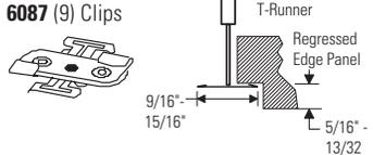
Slotted Grid Ceilings such as Donn Finline and Chicago Metallic Ultraline 3500 and 3600. Use two per 2' and 4' track, three per 8', and four per 12' track.
