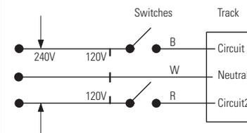
120V 60Hz single branch circuit, 20 amp supply. Maximum load, 2400W (incand.) distributed between track circuits.
