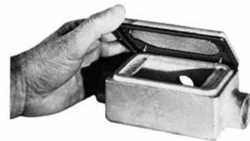
Gasket is designed so that it wraps around ridge top of 0-Z/Gedney aluminum or malleable iron device box. Result is a positive seal against moisture.
