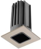
Combined with the driver assembly, the 2 inch aperture recessed downlight is IC rated for insulated or non-insulated applications. Luminaire produces up to 1,000 lumens and is available with optical distributions ranging from 18°- 40°. Low profile form factor allows luminaire to fit in 2 x 6 construction. LED Light Engine provides exceptional fixture to fixture color consistency within a 3-step MacAdam ellipse. Air-Loc rated LED housings and UL Listed for wet location.
