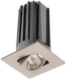
Combined with the driver assembly, the 2 inch aperture recessed adjustable is IC rated for insulated or non-insulated applications. Luminaire produces up to 1,000 lumens and is available with optical distributions ranging from 18°- 40°. Low profile form factor allows luminaire to fit in 2 x 6 construction. LED Light Engine provides exceptional fixture to fixture color consistency within a 3-step MacAdam ellipse. Air-Loc rated LED housings and UL Listed for damp location.
