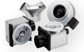
270 CFM fan, two ceiling grilles with lights, two grille housings with dampers, two dimmable 50W halogen bulbs & Y-adapter (4"x 4"x 6"). Uses 4" and 6" ducts. UL Listed for wet locations.
