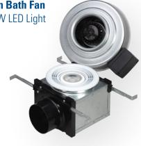
110 CFM fan, one ceiling grille with LED light, grille housing with a damper, dimmable 10W LED bulb. Uses 4" duct. ENERGY STAR® qualified. UL Listed for wet locations.
