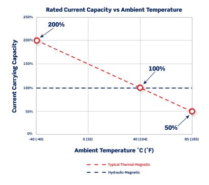
The graph above represents the trip point of a typical Thermal-Magnetic circuit breaker versus a Hydraulic-Magnetic one. Hydraulic-Magnetic circuit breakers are more precise and trip at their marked rating at a wide range of temperature extremes.
