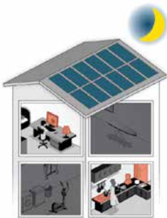
Nighttime: Important loads are powered by the battery
