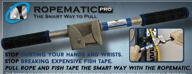
The Ropematic has a durable latch that grabs rope or fish tape when you are pulling down. As you pull back up, the latch loosens and easily slides up the rope or fish tape. You can then pull down again and the Ropematic will grab the rope or fish tape, pulling it down.
