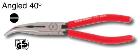
**326 Bent Long Nose Pliers With Cutters DIN ISO 5745** Long nose pliers angled 40°. Extra long cutters for flat and round wire. Partially Serrated Jaws. Cutting edges additionally induction hardened to approx. 64HRC. Special C70 tool steel forgings. Soft vinyl grips are oil & solvent resistant.
