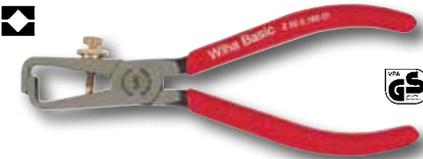
**32645 Stripping Pliers DIN ISO 5744** Heavy duty forged with induction hardened cutting edges for even stripping of insulation. Easy to use adjusting screw allows the stripping diameter to be set. Opening spring for effortless and sensitive handling of pliers. C70 special tool steel. 64HRC cutting edges. For Stripping up to Ø 5mm/#4 AWG conductor cross-section. Soft vinyl grips.
