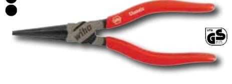
**32633 Long Round Nose Pliers DIN ISO 5745** Extra long head. Serrated Jaws are induction hardened. Special C70 tool steel forgings. Use for gripping and uniform round bending of wires and sheet metal parts. Soft vinyl grips are oil & solvent resistant.
