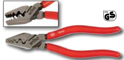
**326 Crimping Pliers DIN ISO 5743** Semi-circular profiles for secure connection between end sleeve and conductor. Long life is achieved through additional induction hardening to 64HRC. C70 special tool steel hardened & tempered. Soft vinyl grips.
