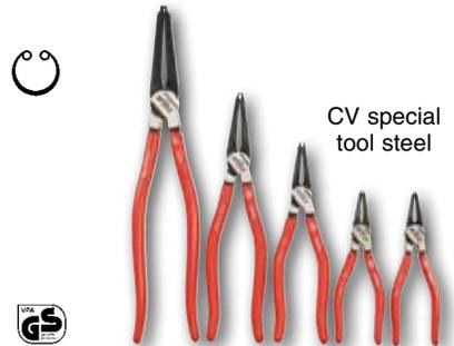
**32626 5 Piece Straight Internal Ring Pliers Set** Shape C, straight tips. Die forged cylindrical precision formed. For inserting & removing internal retaining rings. CV special tool steel.
