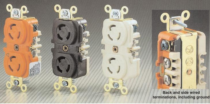
Hubbell Wiring Device-Kellems introduces a new line of duplex Twist-Lock receptacles designed to deliver premium service and long life. This new product design establishes a new standard for 15 amp locking receptacles. A reinforced thermoplastic top and base encapsulate the brass alloy contacts which are locked together by tabs on the mounting strap for
