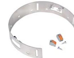
Provides torsion spring mounting capability for 6" housings that do not have torsion spring brackets. 4 pack includes: 4 - retrofit adapter bands, 16 - metal piercing screws, 8 - retrofit lever-action wire nuts
