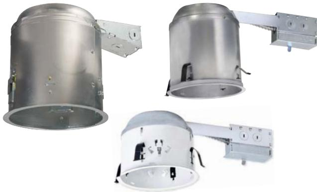
Remodel housings simplify installation when fixtures need to be added to existing ceilings. They can be installed from below in existing ceilings by cutting a precise hole, bringing power to the fixture and installing the housing. The spring clips or speed clamps lock the fixture in place. The integral thermal protector provides positive protection against overlampping. Housings are available in Insulated Ceiling (IC), Non-Insulated Ceiling (Non-IC), Air-Tite (AT) and shallow models.
