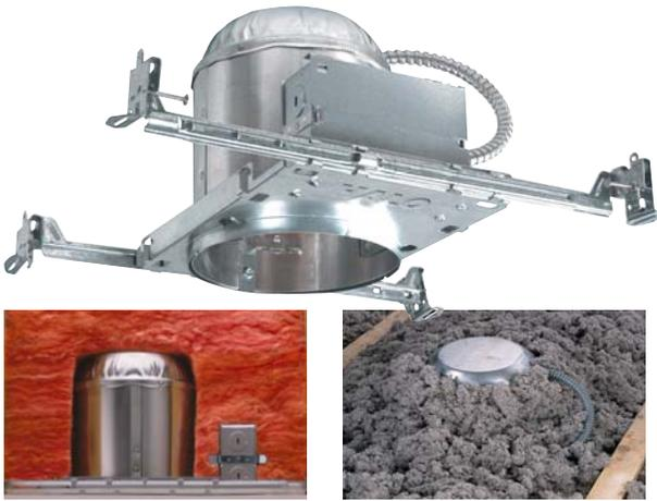
Insulated Ceiling type (IC) rated luminaires are tested to UL 1598 standards for installation with blown-in or batting-type dry insulation materials. This allows the insulation layer to remain unbroken and prevent heating and air conditioning losses. These housings are also equipped with thermal protectors to guard against overlampping by cycling the lamp off and on until the problem is corrected.
