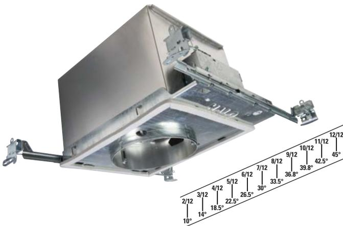
Slope or "cathedral" type ceilings require special housings to keep the lamp aimed straight down rather than following the slope of the ceiling. A lamp aiming mechanism in these fixtures allows the lamp to be aimed vertically in sloped ceilings. Ceiling pitch is measured from 2/12 to 12/12 (the first number refers to the amount of "drop" per 12 inches of horizontal measurement).
