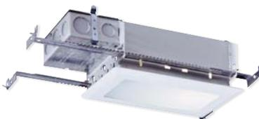
60W A19 lamp. White trim with Albalite diffuser. Junction box rated for feed through branch applications. For non-insulated ceilings. If insulation is present, it must be kept 3" from the fixture on all sides.
