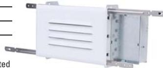
Step light with white louver trim. Fixture is pre-wired to junction box. cULus listed junction box rated for feed through. Integral 120V, 60Hz magnetic ballast. 5W / 7W / 9W Twin Tube 2-pin CFL.
