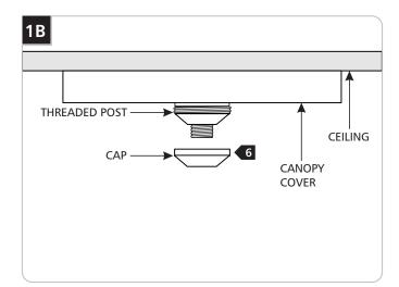
6 Place the canopy cover over the crossbar and screw the cap onto the threaded crossbar post.
