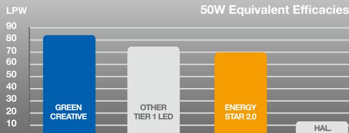
At 83 LPW, this lamp's efficacy is higher than the Tier 1 LED MR16 50W replacement industry average and exceeds ENERGY STAR 2.0 requirements. This energy-saving performance makes this lamp a smart retrofit choice for halogen bulbs.
