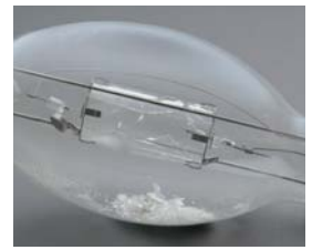
Ruptured arc tube contained within the intact outer jacket of a Venture MP lamp
