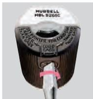
VARI-SIZE® pointer set to "smaller than gauge" position. Cord diameter range is .23 to .36 inch (5.8 to 9.0). Accepts slotted and Phillips head drivers.
