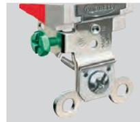
One piece integral grounding terminal with #8 brass screw allows compliance to NEC®. Stainless steel automatic self-grounding clip assures grounding continuity between mounting strap and metal wall box. Steel nickel plated mounting strap provides a corrosion resistant finish.
