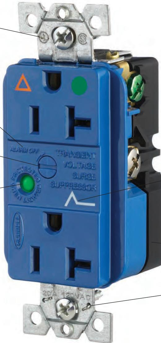
Distinctive surge symbol provides quick visual identification of surge suppression receptacle. High-impact nylon face resists breakage
