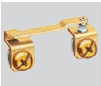
One piece rivetless copper alloy spring contact arm and terminal plate assures proper contact alignment reducing heat rise. Large silver alloy contacts reduce contact erosion and prevent welding, providing long life.
