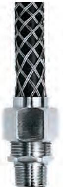
Note: Kellems® Deluxe Cord Grips are suitable for use in hazardous locations per Class I Div. 2, Class II Div. 1 & 2, Class III Div. 1 & 2 of the National Electric Code Sections 501.10(b)(2), 502.10(a)(2), 502.10(b)(2), 503.10(a)(2) and 503.10(b).
