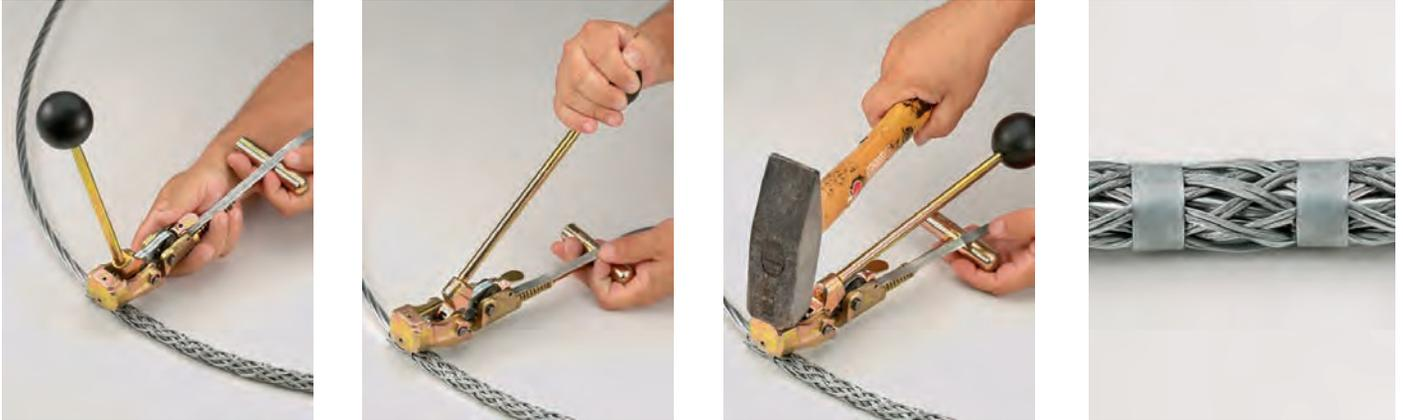
When the tail of a grip is the leading end, the bands are particularly important to prevent accidental release caused by tripping on obstructions. A conductor-to-conductor (double-socking) pulling operation is a good example: where two grips connect two conductors to form a temporary splice. Bands should be applied to the ends of the grips as illustrated herein. It is also common practice to tape over the banded tail area to assure smooth passage through the sheaves.
