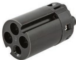
Thermoset polyester contact carrier provides resistance to electrical tracking and withstands higher temperatures. Thermoset properties provide excellent dimensional stability, low moisture absorption, and superior dielectric strength.
