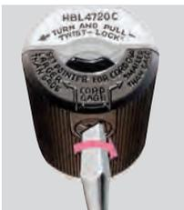
VARI-SIZE® pointer set to "smaller than gauge" position. Cord diameter range is .230"-.360" (5.8-9.0). Accepts slotted and Phillips head drivers.
