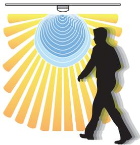
Dual technology occupancy sensors combine both passive infrared (PIR) and ultrasonic (US) technologies for maximum reliability. Because US and PIR need to both detect occupancy to turn lighting on, dual technology sensors minimize the risk of lights coming on when the space is unoccupied—false triggering. Continued detection by only one technology then keeps lighting on as necessary. Dual technology sensors offer the best performance for most applications.
