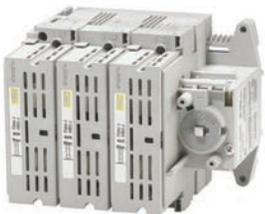
Compact Fused Disconnect Switch accepts Class "J" fuses. Fuse holders are top mounted for easy access. The switch accepts auxiliary contacts for control circuit applications including the ON/OFF control of remote pilot lights or signal for programmable controllers.
