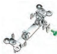
One piece, nickel plated brass mounting strap with integral ground contacts, along with secondary ground contact, provides superior grounding for low resistance flow of fault currents as well as corrosion resistance. Barbed locking arms keep the face locked in place to diminish potential for face/base separation. Back wired ground screw reduces installation time.
