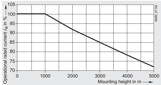
Permissible installation height
