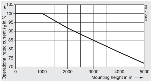
Permissible installation height
