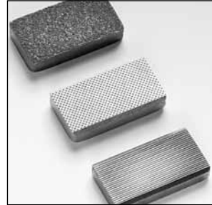
Gripper pads are available in your choice of either parallel, file or grit-type. File-type pads may be used on hard-to-grip insulations such as Kapton® and some Teflon®.
