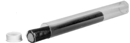
A two part epoxy sealing compound may be used to seal ES sealing hubs. It is quick and easy to measure, mix and install. The compound is kneaded until a uniform color is obtained. It is then packed around the conductors to effectively seal the cable.
