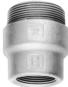
**Note:** Sealing hubs are approved for use in hazardous locations when *Chico*® X fiber and *Chico A* sealing compound are used to make the seal. Sealing hubs are approved for horizontal conduit runs for use in hazardous locations when used with TSC sealing compound, order 1 oz. tube as TSC1.
