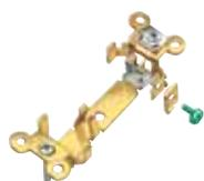
One piece, all brass, mounting strap with integral ground contacts. The safest, most reliable design for a low resistance flow of fault currents. Oversized "bell" shaped ground contacts, along with nickel plated steel retaining shields, help minimize damage to the grounding system during abrupt pullout. Barbed brass locking arms keep the faced locked in place to diminish potential for face/base separation. Back wired ground terminal reduces installation time and increases convenience.
