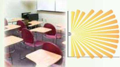
Passive infrared (PIR) technology senses occupancy by detecting the difference between heat emitted from the human body and the background space. PIR sensors require an unobstructed line-of-sight for detection. These sensors utilize a segmented lens, which divides the coverage area into zones. Movement between these zones is interpreted as occupancy. PIR sensors are good at detecting major motion (e.g. walking) and work best in small, enclosed spaces with high levels of occupant movement.
