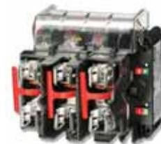
Compact Fused Disconnect Switch accepts Class "J" fuses. Fuse holders are top mounted for easy access. The switch accepts auxiliary contacts for control circuit applications including the ON/OFF control of remote pilot lights or signal for programmable controllers.
