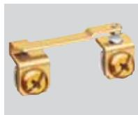
One piece rivetless copper alloy spring contact arm and terminal plate assures proper contact alignment reducing heat rise. Large silver alloy contacts reduce contact erosion and prevent welding, providing long life.
