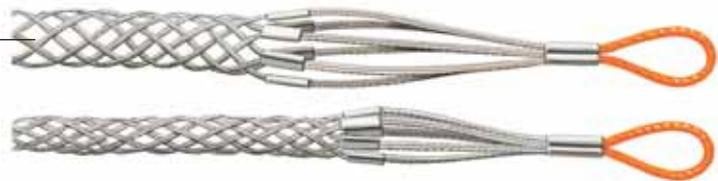
Grips for cable support are easy to install or position. They come in a closed style when the cable end is available, and a split rod style for mid-span installation. Will support the cable's weight as it hangs in vertical, sloping or horizontal position.
