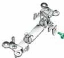
One piece, nickel plated brass mounting strap with integral ground contacts, along with secondary ground contact, provides superior grounding for low resistance flow of fault currents as well as corrosion resistance. Barbed locking arms keep the face locked in place to diminish potential for face/base separation. Back wired ground screw reduces installation time.
