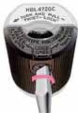
VARI-SIZE® pointer set to "smaller than gauge" position. Cord diameter range is .230"-.360" (5.8-9.0). Accepts slotted and Phillips head drivers.
