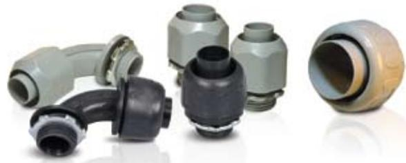
Type NMLT and NMSC nonmetallic connectors are intended to be used with liquidtight nonmetallic conduit Type B; Electri-Flex Types NM and NM2. They are not to be used with Type A (LNM-P) conduit or steel conduit.
