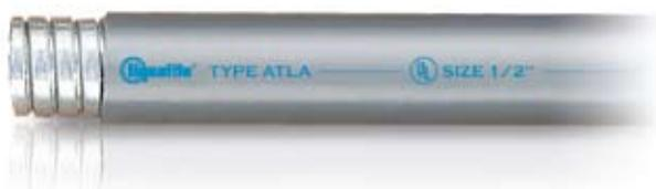
A liquidtight flexible steel conduit designed specifically for extreme hot or cold environments. The flexible inner core is identical to that found in Type LA. The specially formulated PVC jacket remains flexible at low temperatures and resists aging at elevated temperatures. It is listed by Underwriters Laboratories Inc. and certified by Canadian Standards Association.
