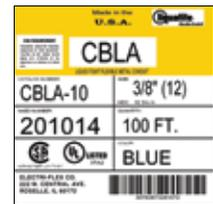
Computer Blue LA (CBLA) is a liquidtight flexible steel conduit commonly used for computer room installations. The blue jacket color easily identifies circuitry for computer power wiring. It is listed by Underwriters Laboratories Inc. and certified by Canadian Standards Association.
