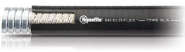
Type SLA is identical to standard UL listed liquidtight flexible steel conduit, but is augmented with a tinned copper shielding braid located over the inner steel core and under its protective PVC jacket. The braid offers a minimum of 90% coverage. Please see the Shielding Effectiveness chart on page 21.
