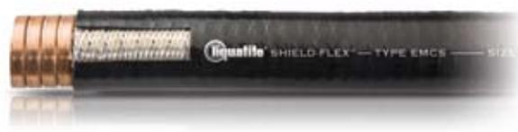
Type EMCS is a hybrid of SLA and EMS. It utilizes the same bronze core and PVC jacket as EMS, but gets further screening protection from a tinned copper braid as found in the SLA product. Please see the Shielding Effectiveness chart on page 21.
