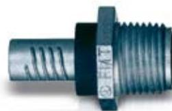
This patented one-piece zinc die-cast liquidtight connector is designed to screw into flexible metallic tubing (FMT). The end of the tubing embeds itself into the rubberized polymer gasket creating a smoke-tight seal as required by the NEC Article 360.40.
