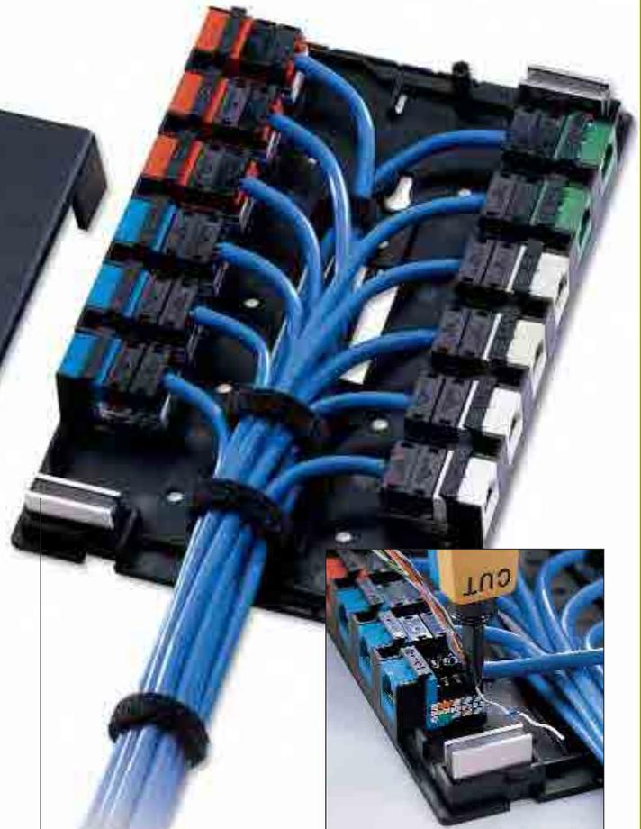
In-port connector termination stations provide stability during punchdown.
