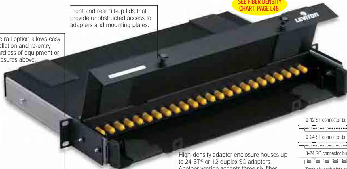
High-density adapter enclosure houses up to 24 ST® or 12 duplex SC adapters. Another version accepts three six-fiber mounting plates; configure with ST, FC, SC, LC and MT-RJ or add a QuickPort plate to create a multimedia enclosure.
