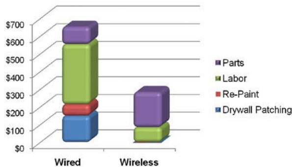
\*Installation time per device: 45-50 minutes for hardwired vs. 10-15 minutes for wireless devices
