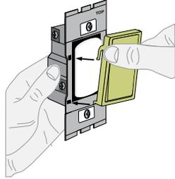
Attach new face by inserting the bottom hinge tabs, then pivot and snap on the new face
