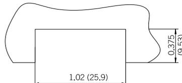
Recommended Panel Opening for Miniature Bi-Pin Snap-In/Slide-On Lampholders
