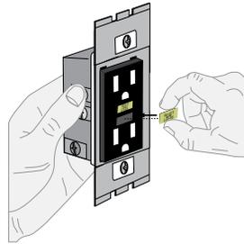
Insert new Test and Reset buttons
