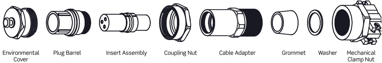
To specify a complete ordering number, select the grommet code from table below and replace “xx”, then select appropriate suffix from the appropriate insert configuration table (see pages **H-38** through **H-43**) and replace “suffix.” Jack Coupling nuts should be used with inserts possessing more than 36 contacts. If environmental cover is not required, replace “E” with “L” in catalog number.
