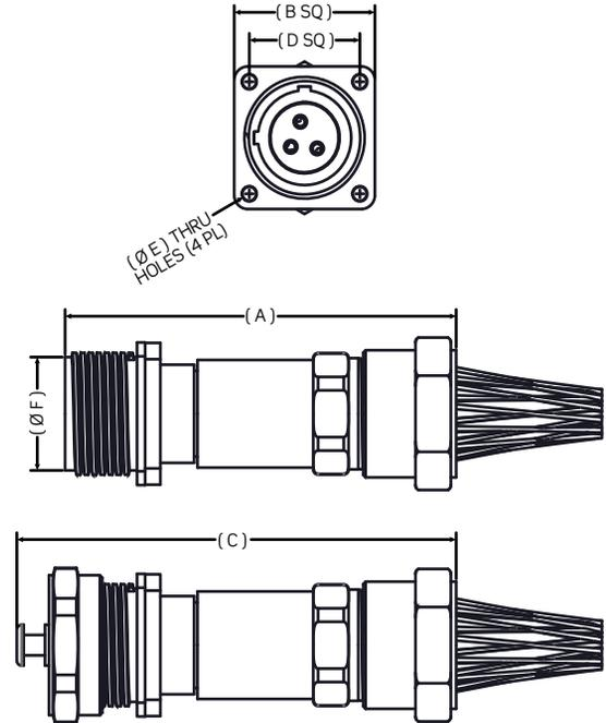
**Square Flange Receptacle With Mechanical Clamp Nut — LZ-REPM Series**
