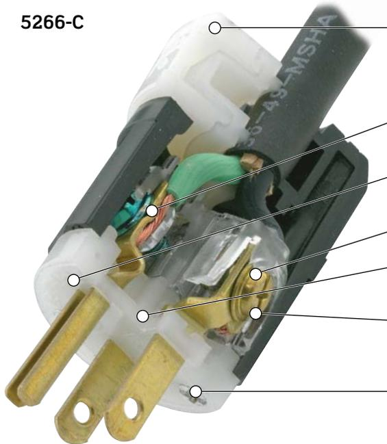
External cord grip utilizes deep triple drive steel screws that are backed out and positioned inside shrouded pockets. External clamps accepts wire mesh grips. Catalog and NEMA numbers printed on cord clamp
