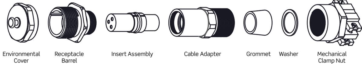
To specify a complete ordering number, select the grommet code from table below and replace “xx”, then select appropriate suffix from the appropriate insert configuration table (see pages **H-38** through **H-43**) and replace “suffix.” If environmental cover is not required, replace “E” with “L” in catalog number.
