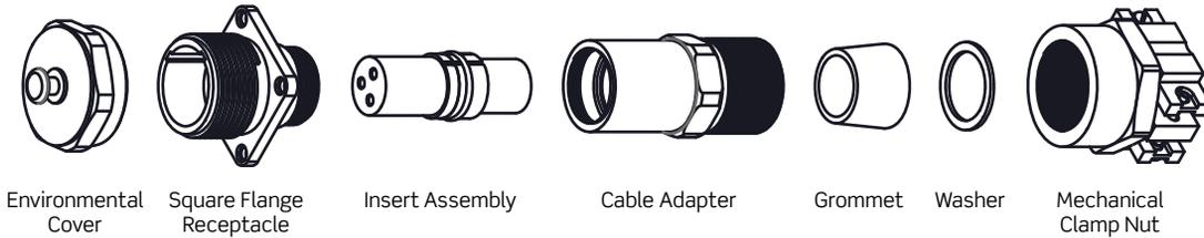
To specify a complete ordering number, select the grommet code from table below and replace “xx”, then select appropriate suffix from the appropriate insert configuration table (see pages **H-38** through **H-43**) and replace “suffix.” If environmental cover is not required, replace “E” with “L” in catalog number.
