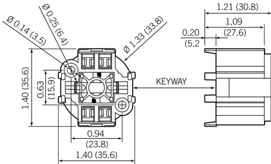
4-Hole Bottom Screw-Down — CFLs 26725-415
