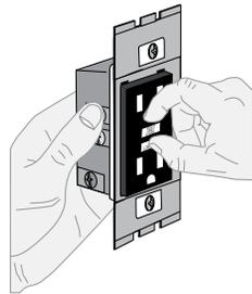
Pull out Test and Reset buttons
