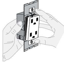
Push down tabs per diagram, one at a time and rotate forward to release face
