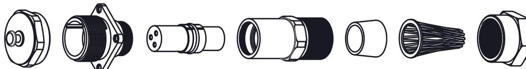
Environmental Cover    Square Flange Receptacle    Insert Assembly    Cable Adapter    Grommet    Basketweave Cable Grip    Gland Nut
