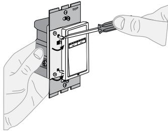
Using a flat screwdriver, push in upper and lower tabs on left side of frame, then rotate right to release face
