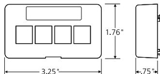
**4-Port Extended Depth Modular Faceplate for installation into shallow raceway channels**
