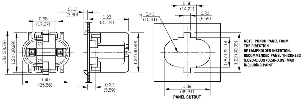
4-Hole Vertical Screw-Down CFLs — 26720-400
