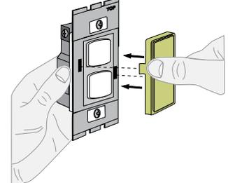
Insert right side tab and rotate left to attach
