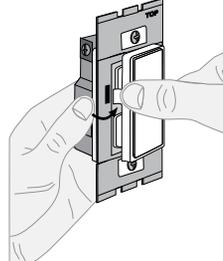
Push in left side of frame at tab and rotate right to release
