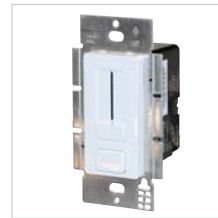
Nora SWITCHEX® All-in-One LED Driver and Dimmer NATL-SWEX100/24 24V 100W Converts 120 VAC to low voltage DC in a standard electrical box. Includes face plate.
