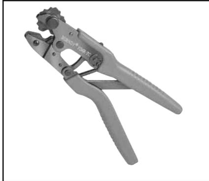
Type Y1MRTC mechanical full cycle ratchet HYTOOL™ will accommodate copper compression HYDENT™ connectors for #8 through #1 code conductor, #8 through #2 Class I flexible strand copper conductor, and #2 solid. The color coded die wheel rotates to provide a proper match of the die and color coded connector. The die index is embossed on the crimped connector for permanent inspectability. A ratchet mechanism assures the tool must complete a full cycle before releasing.
