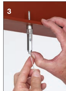
3. Continue pushing through until 1/4" minimum is extending out the side of the KwikWire Hanger
