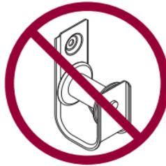
Cable rollers are too expensive and require installation and removal.
