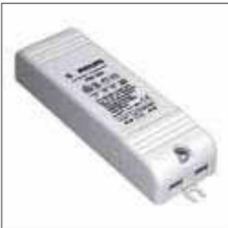
Very low voltage 105 VA dimmable electronic transformer: 230/240 V-12 V-50/60 Hz. Very compact size. Trailing edge-leading edge dimming. Protected against overheating, overloads and short-circuits. Ready to use - quick to install. Min./Max. charge 35 W/105 W. Maximum distance to the lamp 2 m
