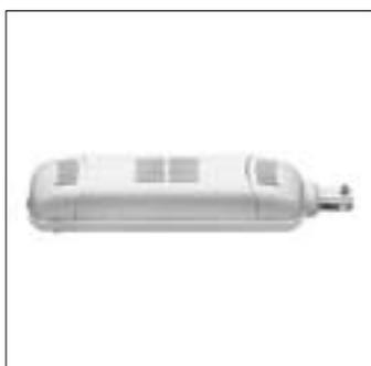
Transformer power supply for direct electrical 12V connection to track. Connection to primary 230V - 240V rated for 150VA, it delivers 11.8V/12.5 A max with protection against short circuits and overloads. Fixing to all surfaces with 2 screws
