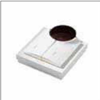
Two-key infrared remote control transmitter for wall mounting and table-top use. The unit can be used in Trios applications. The actual function of the two large keys can be selected with a dip switch in the battery compartment. A dip switch is also used to select the group address.
