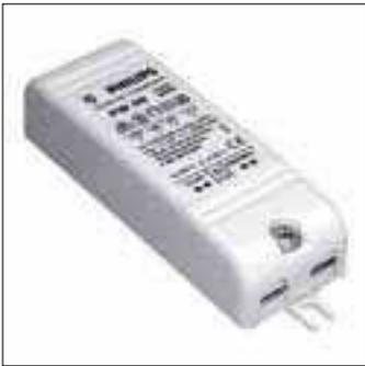
Very low voltage 60 VA dimmable electronic transformer: 230/240 V-12 V-50/60 Hz. Very compact size. Trailing edge-leading edge dimming. Protected against overheating, overloads and short-circuits. Ready to use - quick to install. Min./Max. charge 10 W/60 W. Maximum distance to the lamp 2 m
