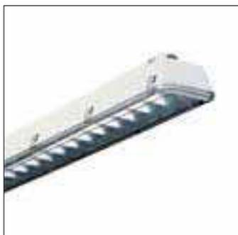
Pacific TCW596 shock-, dust- and jetproof luminaire for TL-D or TL5 fluorescent lamp(s), with OLC semi-high-gloss high-quality aluminum optic with 3D lamellae (D6)
