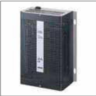
Solo Dimmer; capable of dimming a single channel with total loads of up to 25A. It is suitable for controlling a variety of light sources. The dimmer is controlled by a digital signal, using the DALI (Digital Addressable Lighting Interface) protocol.
