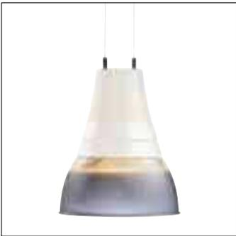
Garnea FPK/KPK/MPK/SPK630 medium-bay luminaire for direct/indirect light distribution, with prismatic reflector; diameter 315 mm (D/I PR)
