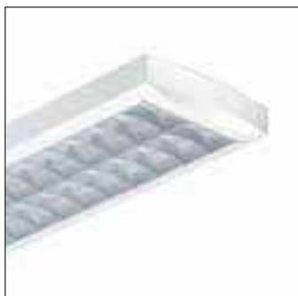
X-tendolight TCS398 surface-mounted basic (BASIC) or line-feature (LF) luminaire with TL5 fluorescent lamp(s) and matt high-quality aluminum optic with profiled lamellae (M2)
