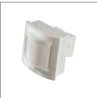
High-bay passive infrared movement detector (mounting height up to 15 m), equipped with an adjustable delay timer (up to 35 minutes). Can be used with all three MDU control units. A dedicated mounting bracket (ZTX400 MB-MDU) is available, into which the movement detector can be clicked.
