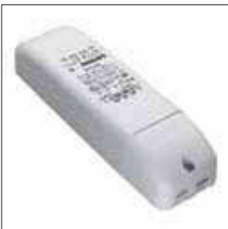
Very low voltage 150 VA dimmable electronic transformer: 230/240 V-12 V-50/60 Hz. Very compact size. Trailing edge-leading edge dimming. Protected against overheating, overloads and short-circuits. Ready to use - quick to install. Double terminal block on the 230 V primary circuit. Triple terminal block on the 12 V secondary circuit.
