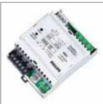
The 1 - 10V Converter has been designed to control HF-R ballasts. This ensures that MultiDim systems are compatible with and easily integrated into existing systems. The converter can switch a maximum of 12 HF-R ballasts. The analogue 1 - 10V signal and the digital DSI signal can control 50 HF-R ballasts.
