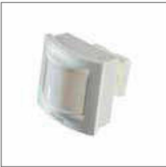
Wall-mounted passive infrared movement detector for energy-saving solutions in indoor lighting applications. It detects movement within an angle of 90° (maximum range 15 m at a mounting height of 2.1 m). Adjustable switch-off delay time of up to 35 minutes. Electrical connections via an additional sensor cable with a modular
