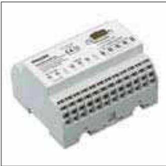
Individually control up to 48 RGB luminaires with one of the four pre-programmed sequences or create your own dynamic sequence. You can create the sequences with Windows-compatible software and upload via a standard serial connection. Individual control of up to 144 DMX channels
