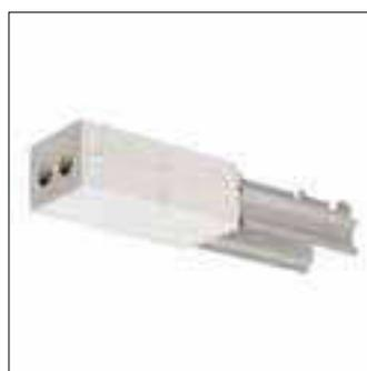
The continuous-line connection unit is used at the end of a light-line when a through-connection is needed to pass an interruption of the light-line. It comprises a 7-pole screw connection block. The same continuous-line connector is used for the TTX400 with either the internal 5- or 7-wire flat ribbon cable. Not to be used for
