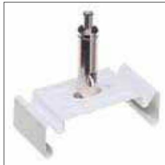
Cable suspension bracket for suspending the TTX400/410 sections from steel cable M 1.8. Integrated clasp mechanism allows easy, tool-less adjustment of the mounting height. Steel cable can be ordered separately with accessory ZTX400 SW1.8-10000
