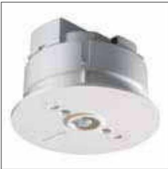
Occuswitch advanced version. LRM1080 is a movement detector with a built-in switch. It switches the lights off in a room or area when it is vacated, thus saving up to 30% on electricity consumption. Occuswitch can switch any load up to 6 A and control an office area of around 20 m<sup>2</sup>. A detachable mains connector
