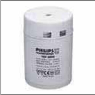
Very low voltage 50 VA toroidal transformer: 230 V-12 V-50/60 Hz. Protected against overheating, overloads and short-circuits. Ready to use - quick to install. Opening cap. Automatic cable holder. Automatic secondary connection. Self-screwable base. Unlockable baseplate. Minimum charge 20 W
