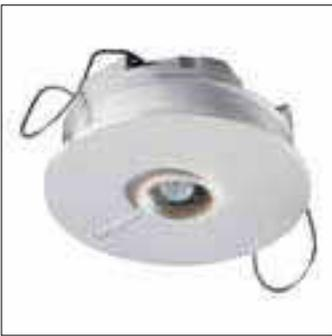
Compact advanced movement detector that features variable delay-to-off via DIP switch and can be part-shaded to limit coverage. The sensor is powered via the additional modular plug-in (RJ12) connector cable that attaches it to a lighting controller. The sensor is suitable for both recessed and surface mounting. Mounting height is
