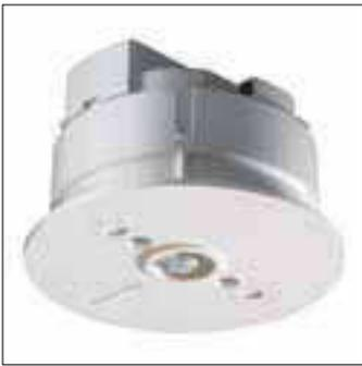
Occuswitch basic version. LRM1070 is a movement detector with a built-in switch. It switches the lights off in a room or area when it is vacated, thus saving up to 30% on electricity consumption. Occuswitch can switch any load up to 6 A and control an office area of around 20 m<sup>2</sup>. A detachable mains connector enables
