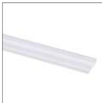
Cable duct, for installing on the trunking, in white plastic, with a length of 2 or 3 electrical units. Can be closed with blind cover strips. To be used in combination with the suspension brackets ZTX400 UCD/CCD. Also available in length of 49, 54 W.
