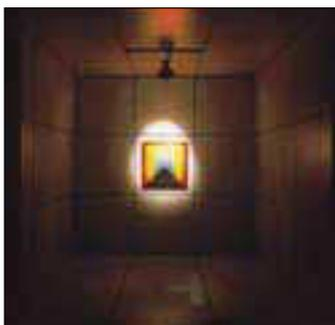
K2 is a spot which stands out due to its sharp transition to a minimal amount of spill light; this type of beam is excellent for creating theatrical and dramatic effects. This class is usually associated with very high-intensity beams.
