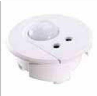
This ceiling-mounted multi-sensor contains an IR receiver, a constant light sensor that measures reflected light from below the device, and a PIR occupancy sensor. The multi-sensor is provided with a 40° angle restrictor for the light sensor. The timer of the PIR occupancy sensor can be set between 1 and 85 minutes.
