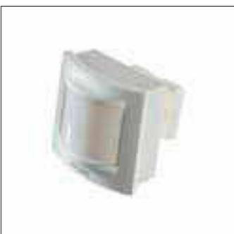
Wall-mounted passive infrared movement detector for energy-saving solutions in indoor lighting applications (automatic light switching based on occupancy). It detects the slightest movement within a range of 25 m. Adjustable switch-off delay time of up to 35 minutes. Electrical connections via an additional sensor cable with a
