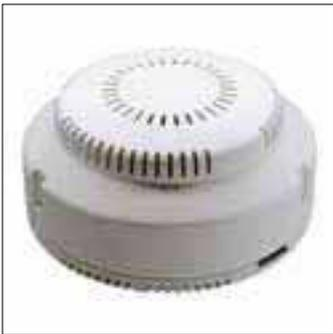
Very low voltage 310 VA toroidal transformer: 230 V-12 V-50/60 Hz. Protected against overheating, overloads and short-circuits. Ready to use - quick to install. Single terminal block on the 230 V primary circuit. Triple terminal block on the 12 V secondary circuit. Self-screwable base. Unlockable baseplate. Minimum charge 20 W
