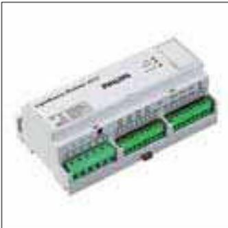
DIN-rail unit with 4 separate outputs (Switching & Regulating [1-10V]) able to switch a load of 5 A each to control luminaires directly or via contactors in the cabinet to switch higher lighting loads.
