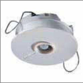
Compact movement detector to be used to expand the detection area of luminaires incorporating ActiLume. The sensor is connected to the DALI bus from the ActiLume luminaire and does not require external power. The sensor is suitable for both recessed and surface mounting. Mounting height is between 2.5 and 3.5 m.
