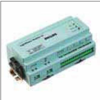
Input unit with 4 sensor interfaces (light sensors, movement detectors and infrared [IR] receivers) and 4 inputs for standard wall switches/emergency test sensors. DIN-rail unit, which is also suitable for use as an installation box, i.e. this unit does not require an outer enclosure.
