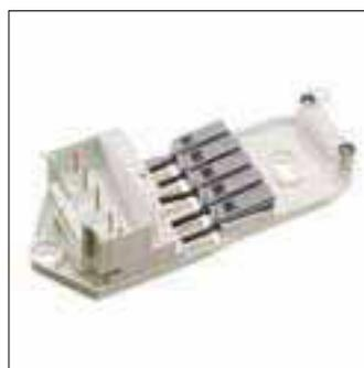
Electrical connector for attaching waterproof and surface-mounted luminaires to the prewired trunking TTX400. This electrical connector can be clicked on the connection block as mounted standard in the TTX400 light-line (also ZTX400 DC). The electrical connector comprises insert contacts and a strain reliever
