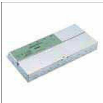
Lighting Control Module with 4 volt-free outputs, Switching & Regulating (1-10V), to allow separate circuits of the same phase to be switched. There are 2 permanent supplies for emergency luminaires, also volt-free but switched simultaneously. The 4LS has 4 sensor interfaces (light sensors, movement detectors and infrared [IR] receivers)
