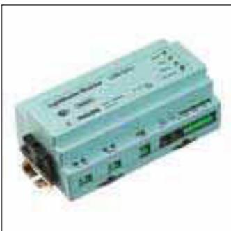
DALI Lighting Control Module in a DIN-rail housing with 1 DALI output. This controller can switch and regulate up to 64 DALI devices. The DALI devices can be controlled separately or in groups. The unit has inputs for sensors and switches, but is designed to work in combination with the 4SI input unit for sensors. The use of
