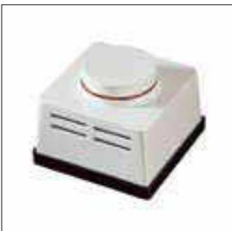
Manual rotary potentiometer with microswitch for surface mounting. In combination with one or more electronic 1-10V HFR ballasts, electronic light regulators or Trios controllers, it serves to control the light level of fluorescent lamps, halogen lamps or incandescent lamps.
