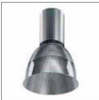
Pendola CPK/FPK/HPK/MPK/SPK440 high-bay pendant luminaire with prismatic reflector; diameter 410 mm, wide beam (P-D410-WB)
