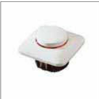
Manual rotary potentiometer with microswitch for recessed mounting. In combination with one or more electronic 1-10V HFR ballasts, electronic light regulators or Trios controllers, it serves to control the light level of fluorescent lamps, halogen lamps or incandescent lamps.
