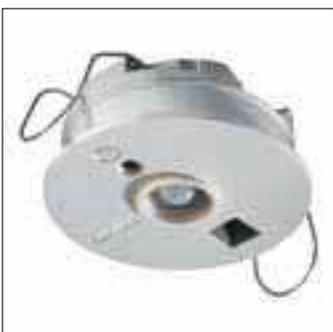
Compact multi-sensor combining advanced internal light sensor, movement detector and infra-red receiver. The unit features individual element selection, variable delay-to-off via DIP switch and auto-calibrating light sensor. The movement detector can be part-shaded to limit coverage. The sensor is powered via the additional
