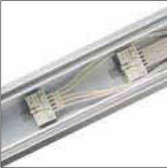
Maxos 4MX656 TL5 and 4MX056 TL-D standard trunking section with two 5-wire flat ribbon cables (2x5x1.5/2x5x2.5); to create different zones in an application or use central emergency systems
