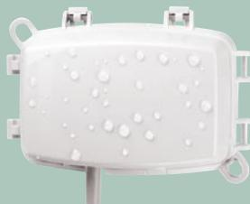
These NEMA 3R receptacle covers ensure compliance with 2005 NEC Article 406.8 (B) (1) which requires that 15 and 20 ampere, 125 and 250 volt receptacles installed in a wet location have an enclosure that is weatherproof whether or not the attachment plug cap is inserted. They also meet the 1999 NEC Article 410-57(b) and are designed to meet the 1999 NEC Article 210-60(b), which requires that receptacles installed behind beds in hotels and motels be protected with a suitable guard.
