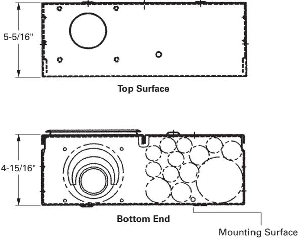
**Semi-Flush Stucco Unit Knockout Configurations and Dimensions for MBE2040B200BTS, MBE2040B225BTS, MBE2040B200BTF and MBE2040B225BTF**
