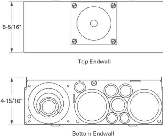
**Knockout Configurations and Dimensions for Catalog Numbers MBT48B125BTS, MBT48B150BTS, MBT48B200BTS and MBT48P200BTS**
