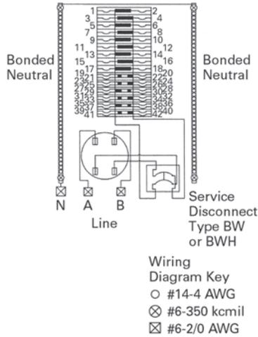
**Typical Wiring Diagram for Catalog Numbers MBED2040B200BFN, MBED2040B225BFN**
