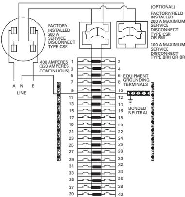
Type BR Wiring Diagram Key
