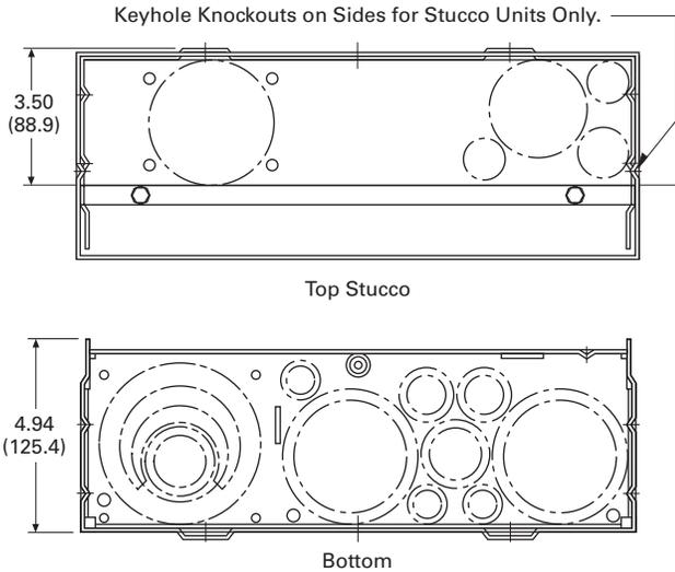
**Knockouts for Stucco and Surface Units Catalog Numbers—MBE1224B100TS, MBE1224B125TS, MBE816P200TS, MBE816P200TSCU, MBE2040B200TS, CMB1212P200BTS, CMB1212P200BTSD, CMB1212B200BTS, MB1212L200BTS and CMB1212L200BTS**
