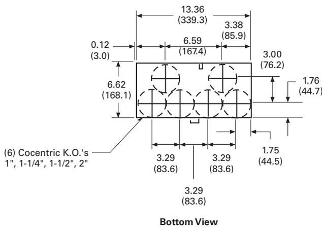
**Note:** Dimensions Apply to 800 and 1200 Ampere Horizontal Bus.
