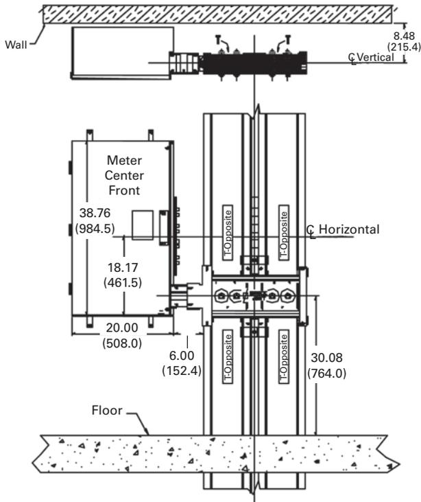
**Main Circuit Breaker—“Standard T” Phasing Right**
