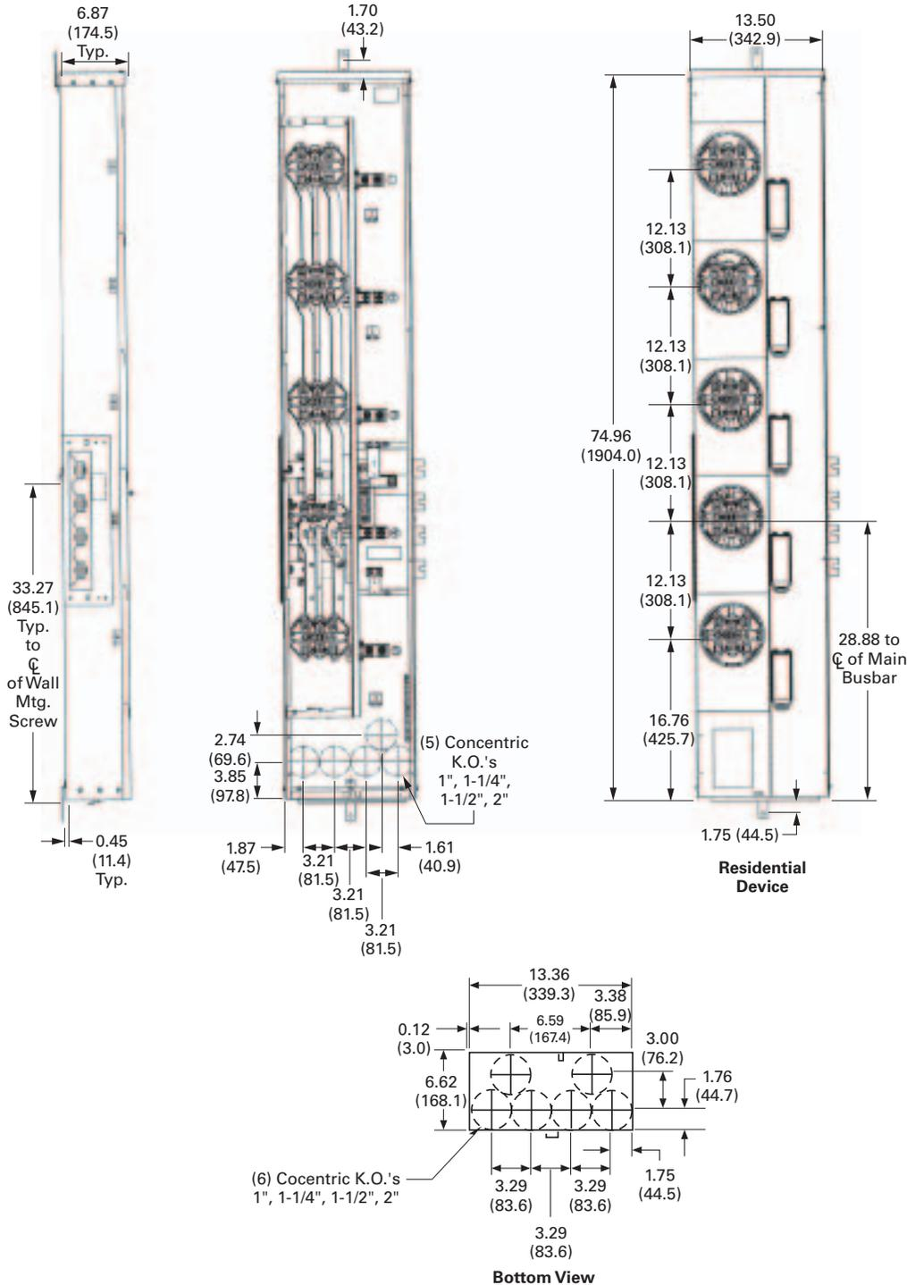
**Note:** The Bussed meter stack device shown on the far right of the figure, must be used on Mains with Busway connections, found on **Pages V1-T4-109 and V1-T4-113**. Please contact factory for catalog numbers associated with Bussed meter stack devices.
