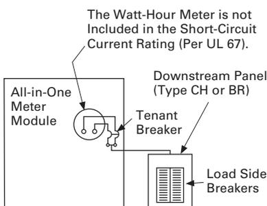
**Note:** The ratings for both 125 and 200 A tenant positions apply to both Type BR and CH loadcenters and 10 kAIC branch breakers.
