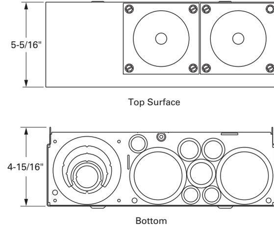
**Surface Unit Knockout Configurations and Dimensions for MBE2040B200BTS, MBE2040B225BTS, MBE2040B200BTF and MBE2040B225BTF**
