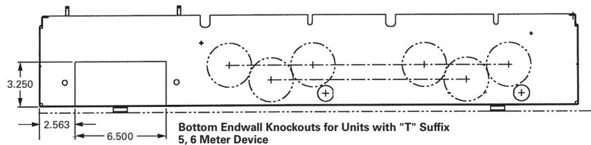
Bottom Endwall Knockouts for Units with "T" Suffix
