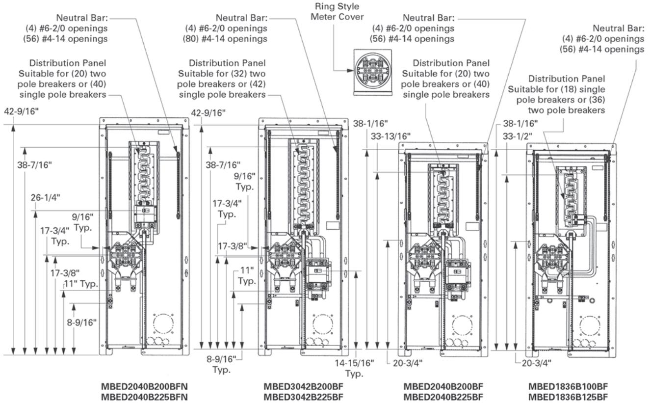
Knockout Configurations and Dimensions for MBED2040B200BFN, MBED20408225BFN, MBED3042B200BF, MBED3042B225BF, MBED2040B200BF, MBED2040B225BF, MBED1836B100BF, MBED1836B125BF
