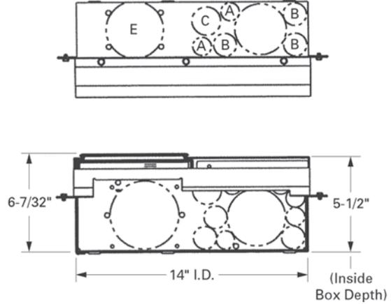
**Knockout Configurations and Dimensions for Catalog Numbers CMBXP200BTS, CMBXB200BTS, CMBX1212P200BTS and CMBX3242P200BTS, CMBX3242B200BTS, CMBX1212B200BTS**
