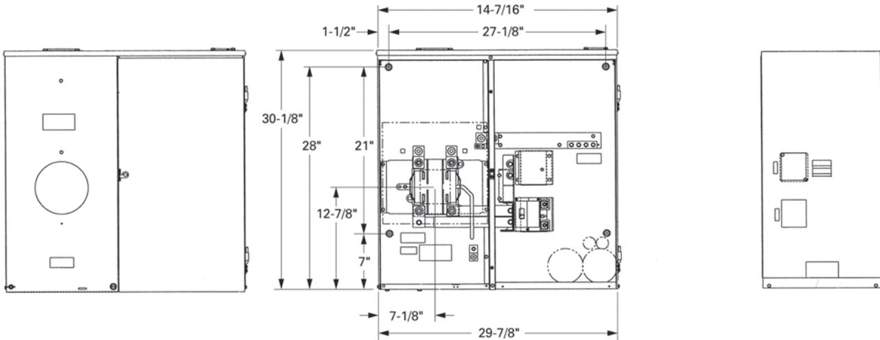
Knockout Configurations and Dimensions for HPC40SHL and HPC30SHL
