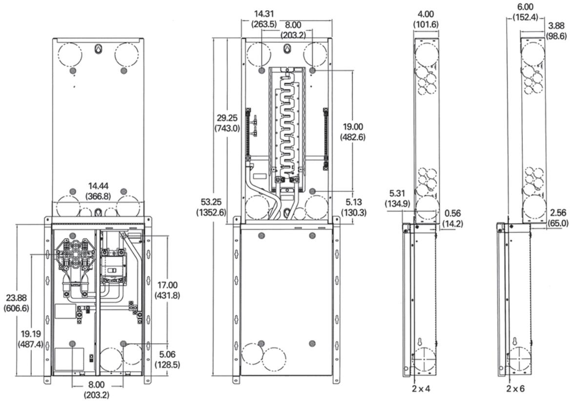
Knockout Configurations for MBEB2003040BB, MBEB2253040BB
