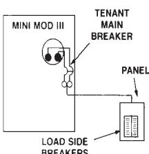
GE breakers rated 10,000 AIC or greater when installed on the load side of Mini Mod III are protected for the interrupting rating per the UL Listing marked on the tenant breaker.
