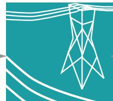
**Power lines** branch off and feed the power through **step-down transformer substations** for local distribution. **Pole-mounted transformers** step down the voltage to 120 volts for delivery to your home.
