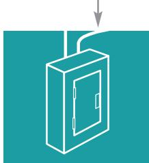
**Main lug load centers**, or subpanels, supplement the load center and allow the addition of branch circuits to the home's electrical system.
