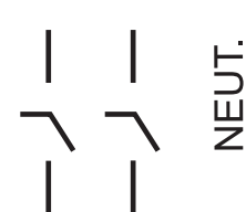
Three-wire SN, 120/240 Volts AC, No Fuse
