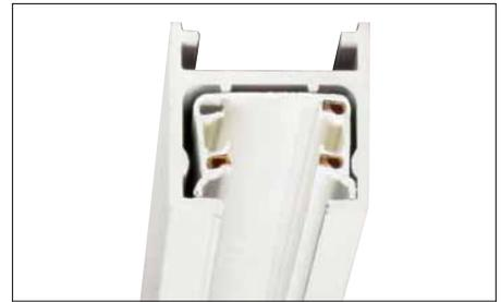
Advent double-circuit track allows for separate control of the Lytespots on the same track. It can be surface or stem mounted on ceilings, and mounted vertically or horizontally on walls, in straight runs or patterns. It can be field cut to the desired length. Total capacity is 40 amps when supplied by a single phase, 120/240V three-wire branch circuit.
