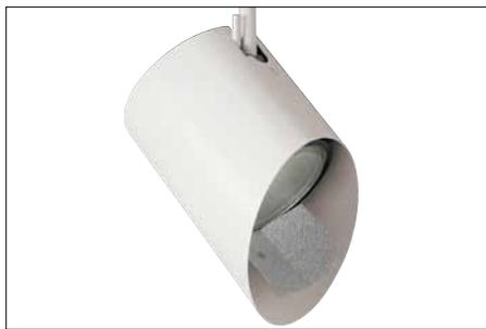
ProSpec Wall Washers feature an asymmetrical spread lens and an anodized aluminum kick reflector to distribute light evenly from ceiling to floor. The kick reflector assembly can hold one accessory and be removed from the front for relamping. ProSpec's Tru-Lock™ aiming mechanism allows simultaneous locking of both horizontal and vertical positions. Ring Wall Washers feature highly adjustable yoke mounting.
