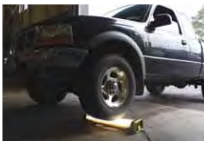
K&H Tuff! Above, the Quad Light undergoes K&H extreme product testing for durability and shatter resistance.
